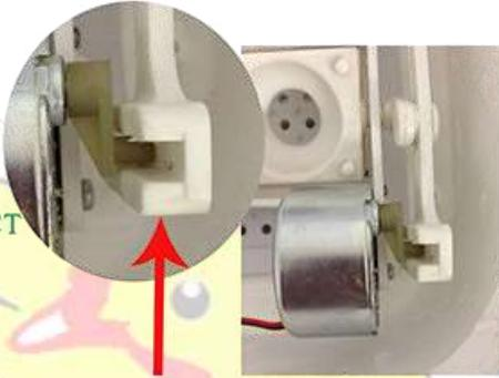
Gearbox's shaft must be in its place for turning the egg trays
