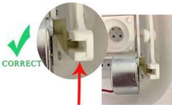
Gearbox's shaft must be in its place for turning the egg trays
