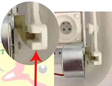
Gearbox's shaft must be in its place for turning the egg trays
