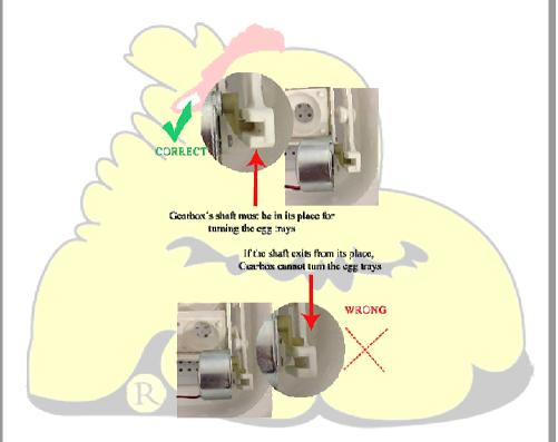
Turn the machine on and note the following:
