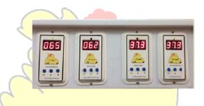
In normal situation main controllers work and set the temperature and humidity.
